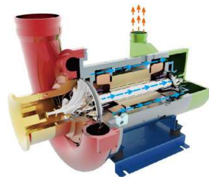
Motor Cooling System
